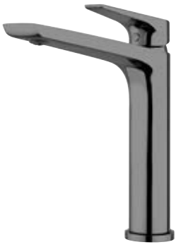
SOLITAIRE Sink Mixer Mirrored Black SLT11MB AP PVD 10 W Min. Pressure 35kPa WELS: Mains 3 Star; 8L/min Low/Unequal 5 Star; 6L/min 360° Swivel Spout
