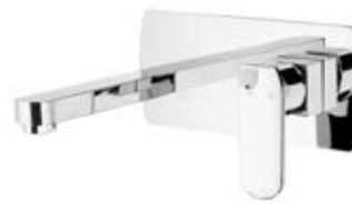
FUSION Wall Mounted Basin & Bath Mixer Chrome FSN9 MP 10 Min. Pressure 150kPa WELS: Mains 3 Star; 8.5L/min Low/Unequal 2 Star; 11.5L/min Spout reach: 190mm
