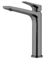
SOLITAIRE Sink Mixer Mirrored Black AP PVD 10 W Min. Pressure 35kPa WELS: Mains 3 Star; 8L/min Low/Unequal 5 Star; 6L/min Product code: SLT11MB
