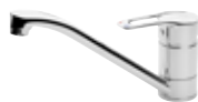
FORENO Loop Lever Sink Mixer Chrome AP 10 Min. Pressure 35kPa WELS: Mains 4 Star; 7L/min Low/Unequal 2 Star; 11L/min Large bore hot hose and port Product code: FMX2.1
